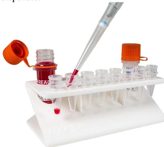
**Figure 3: Dispensing BCC19 Reagent 1 into MD-Bio PCR Strip**
